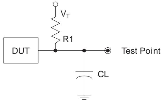
**Table 10-1. Test Fixture Required Components, Non-Terminated Interfaces**
