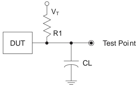
**Table 3-3. Test Fixture Required Components, Non-Terminated Interfaces**
