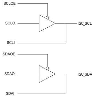
To use the dedicated I2C pins, start by instantiating or inferring the IO buffer. The I2C\_SCL or I2C\_SDA are then assigned to the dedicated pins unless the dedicated pins are not available. Note that the I2C pins do not have to use the dedicated pins. Refer to Figure 21-4 for the routing connections.
