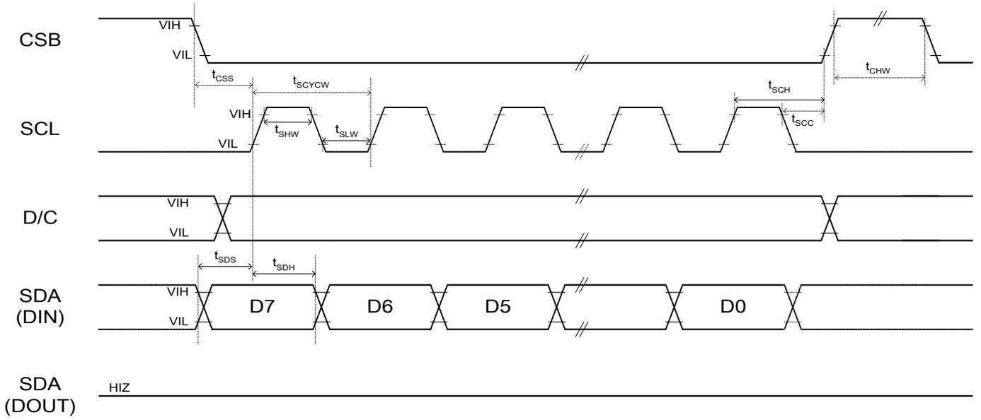
Note 7-6. 4 pin serial interface characteristics (read mode)
