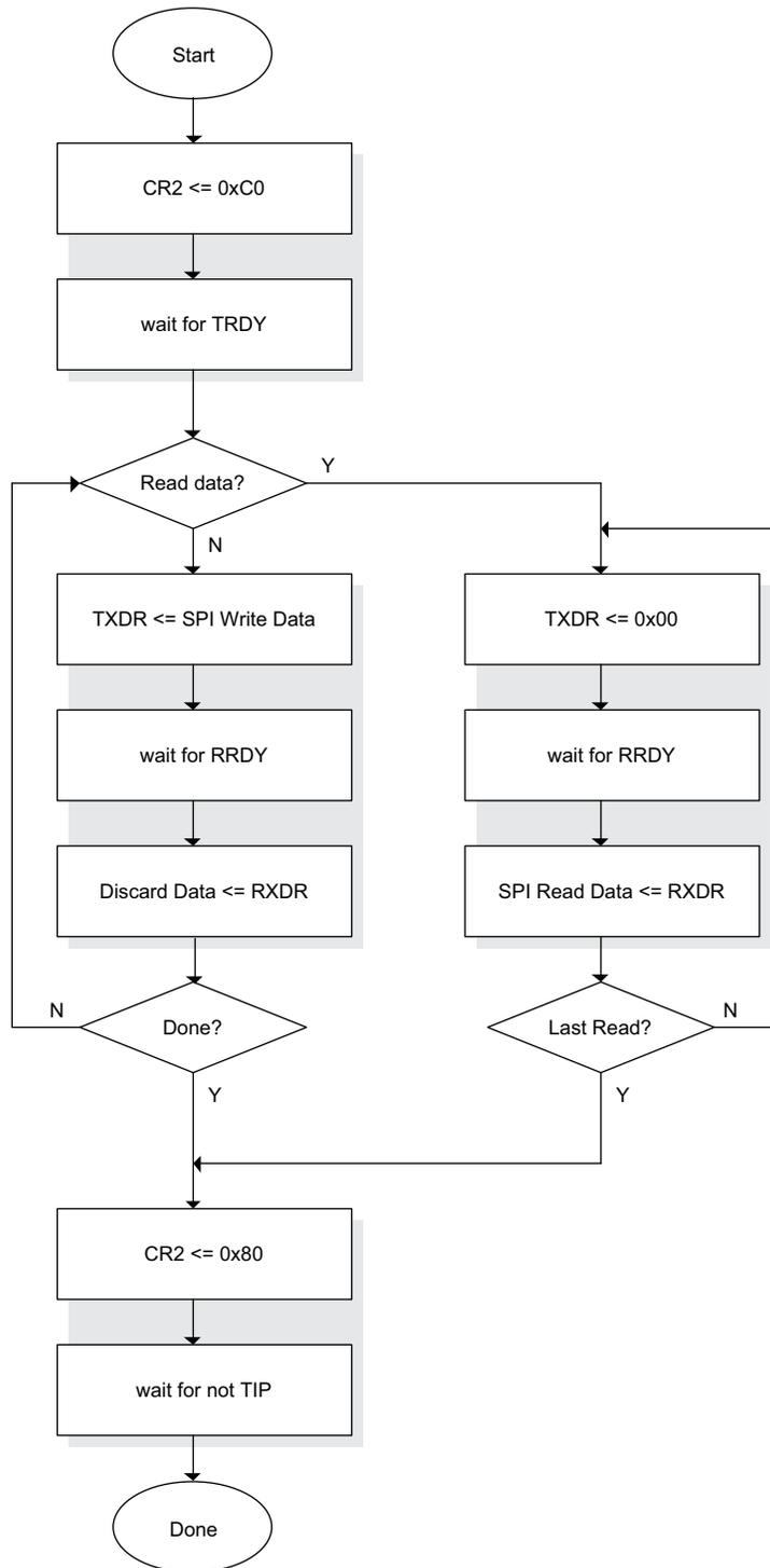
*Note: Assumes CR2 register, MSCH = '1'. The algorithm when MSCH = '0' is application dependent and not provided. See Figure 22-15 for guidance.*
