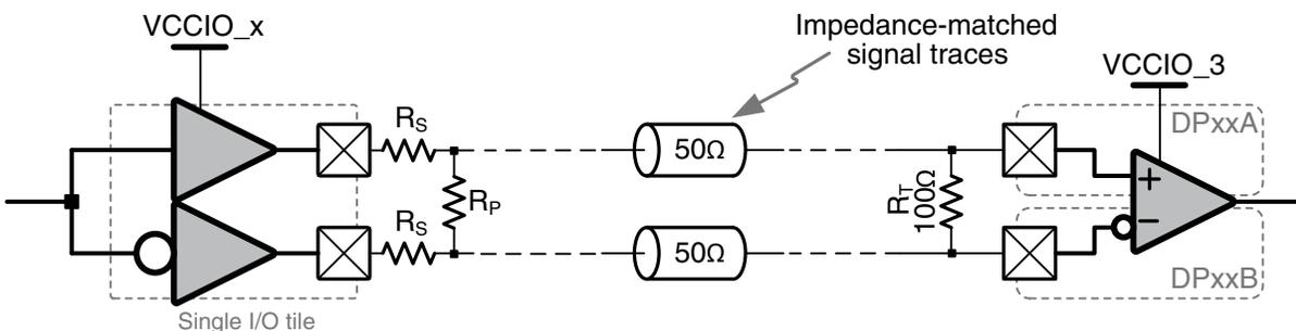
The resistor values for the compensation network are described below. These equations are also provided in the Differential I/O spreadsheet. The variables are defined and described in Table 19-2.
