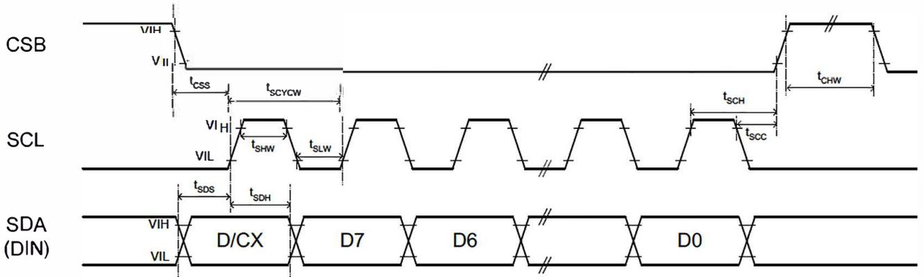
Note 7-4. 3 pin serial interface characteristics (read mode)
