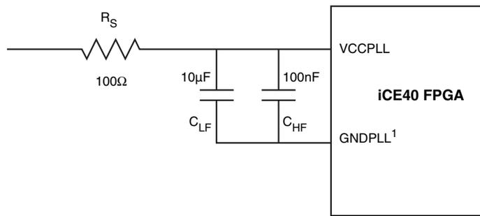
1. Note that GNDPLL should not be connected to the board's ground.
