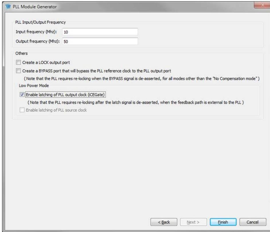
After selecting the desired values, the final window the PLL Module Generator opens, as shown in Figure 17-10. This window shows all the values of the attributes and parameters that were discussed in the previous sections and in Tables 17-4 and 17-5. It also shows which PLL Macro type has been selected. The PLL Macro Type used in this example is SB\_PLL40\_Core.
