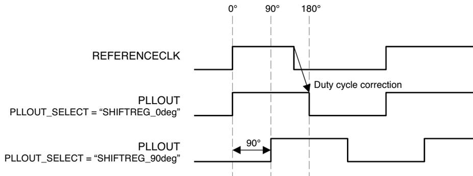
Unlike the Fine Delay Adjustment, the quadrant phase shifter always shifts by a fixed phase angle. The resulting phase shift, measured in delay, depends on the clock period and the PLLOUT\_PHASE phase shift setting, as shown in the equation below.
