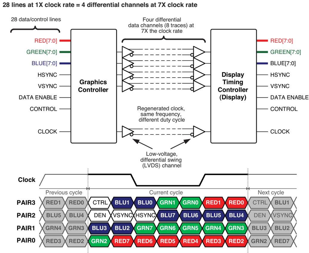
At the receiving end, the differential data is de-serialized and converted back into a wider bundle of single-ended signals.
