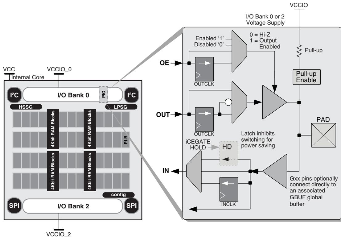
The PIO contains three blocks: an input register block, output register block iCEGate™ and tri-state register block. To save power, the optional iCEGate™ latch can selectively freeze the state of individual, non-registered inputs within an I/O bank. Note that the freeze signal is common to the bank. These blocks can operate in a variety of modes along with the necessary clock and selection logic.
