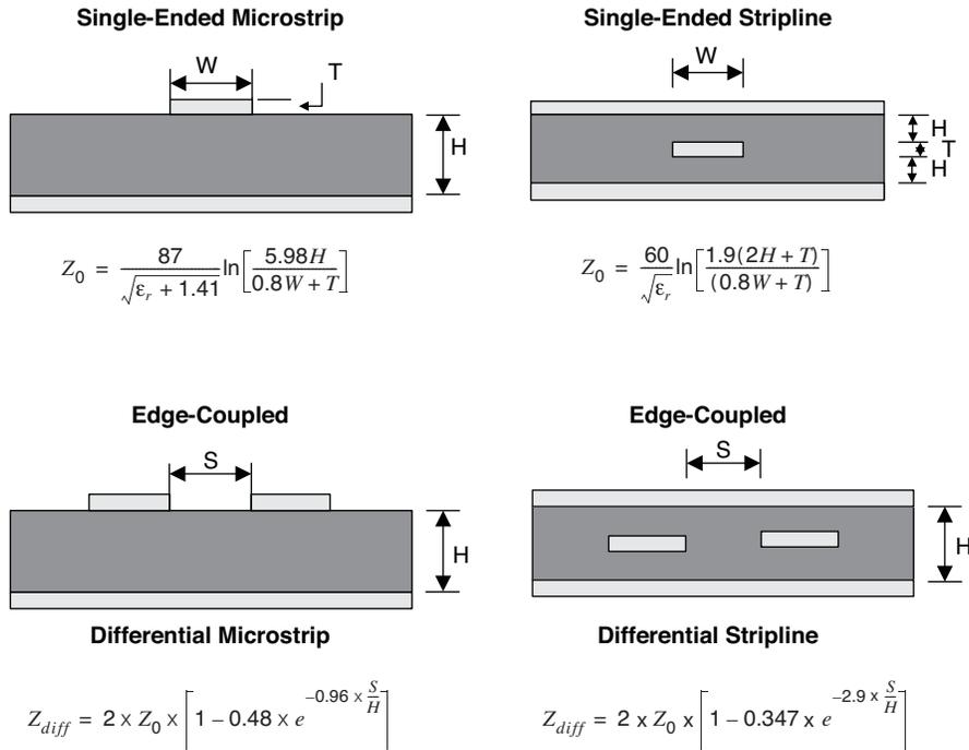
Typical PC board trace impedance is  $Z_0 = 50\ \text{Ohms}$ . For a single-ended microstrip, the trace impedance is calculated by using the following equation:
