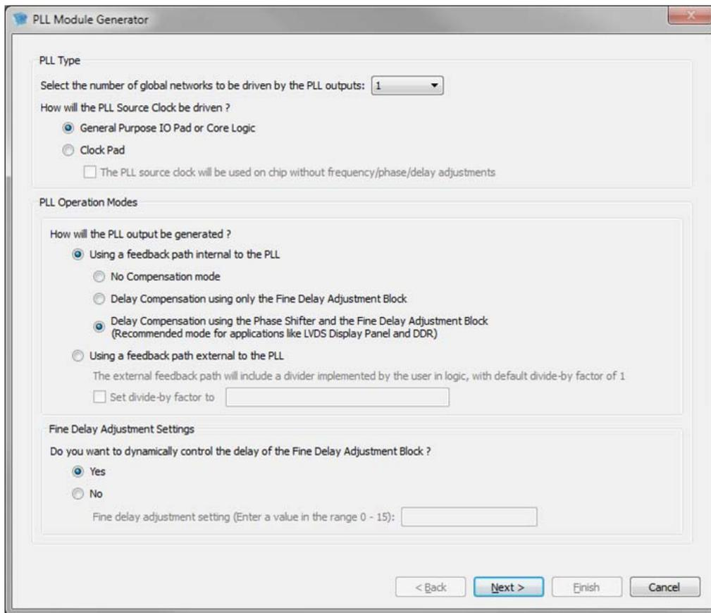
Refer to Table 17-8 for details on user options. Select desired settings which are self-explanatory. Note that some of the options are only activated when other required selections are made. These settings directly modify the PLL signals and attributes of the PLL software macro, as explained in Tables 17-4 and 17-5.
