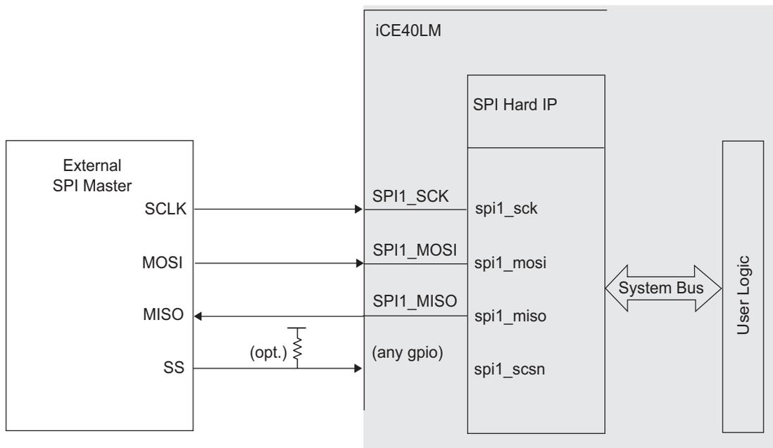
2. iCE40LM User SPI Master accessing one or multiple External Slave SPI devices
