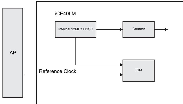
The calibration circuit for strobe generator can be improved for the purpose of power saving as shown in Figure 20-3.
