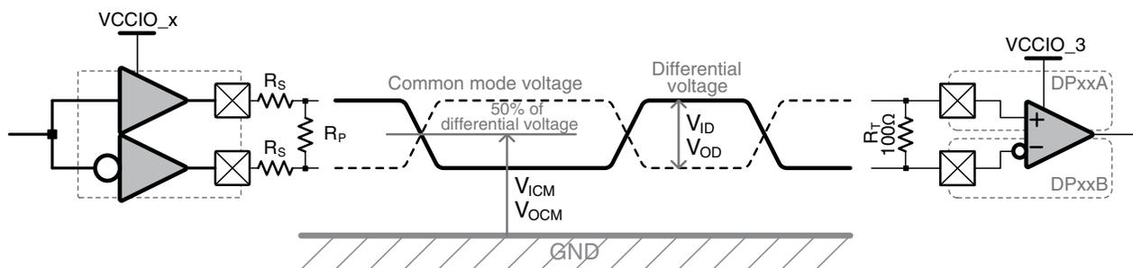
The key electrical parameters are the common mode voltage and the differential voltage. For iCE40™ applications, the common mode voltage is essentially half the I/O Bank supply voltage. The differential voltage depends on the values of the external compensation resistors, discussed in “[LVDS and Sub-LVDS Termination](#)” on page 3.
