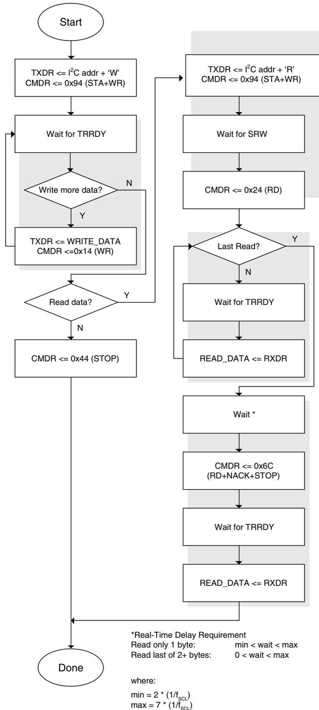
Figure 22-6 shows a flow diagram for reading and writing from an I2C Slave device via the System Bus interface.
