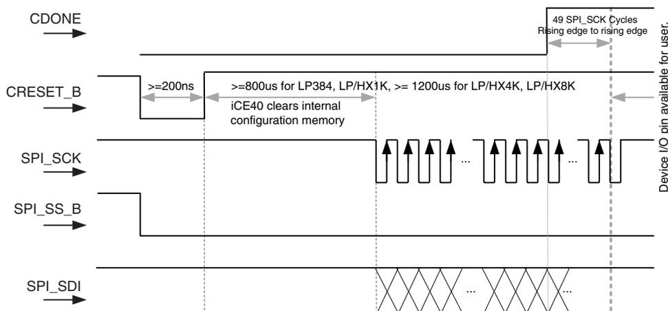
Figure 15-15. iCE40 Timing Waveform 2
