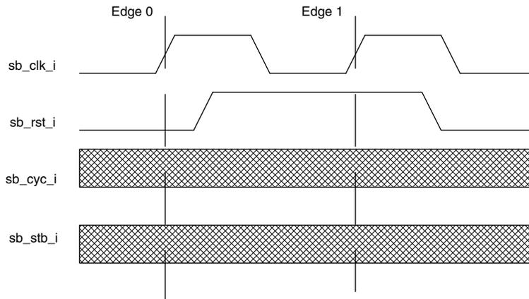
The sb\_rst\_i signal can be asserted for any length of time.
