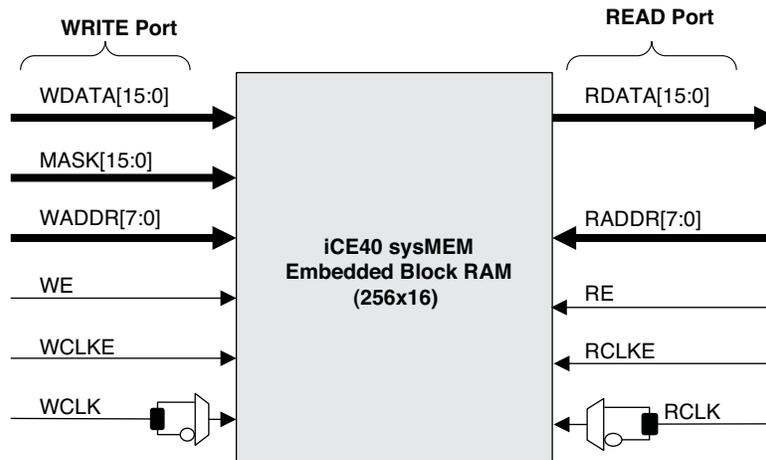
Using programmable logic resources, an EBR implements a variety of logic functions, each with configurable input and output data widths.
