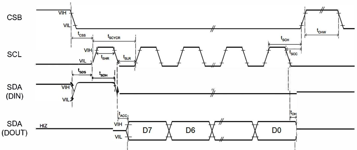
Note 7-5. 4 pin serial interface characteristics (write mode)
