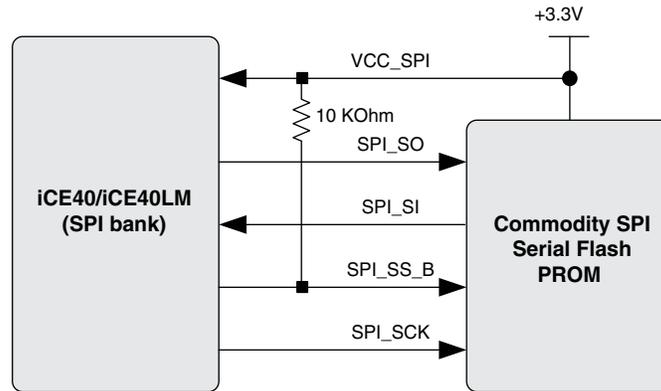
The SPI configuration interface is used primarily during development before mass production, where the configuration is then permanently programmed in the NVCM configuration memory (only available in iCE40 LP and iCE40 HX devices). However, the SPI interface can also be the primary configuration interface allowing easy in-system upgrades and support for multiple configuration images.
