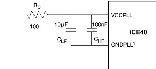
1. GNDPLL should not be connected to the board's ground
