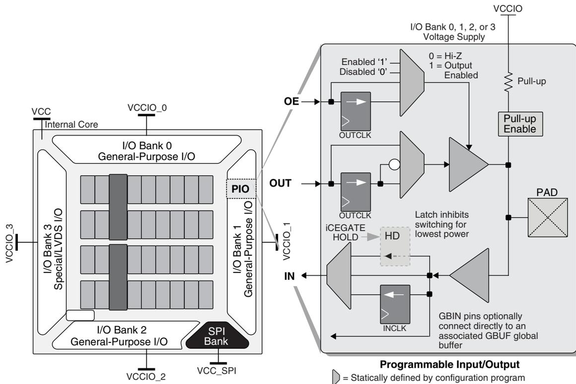
The PIO contains three blocks: an input register block, output register block iCEgate™ and tri-state register block. To save power, the optional iCEgate™ latch can selectively freeze the state of individual, non-registered inputs within an I/O bank. Note that the freeze signal is common to the bank. These blocks can operate in a variety of modes along with the necessary clock and selection logic.
