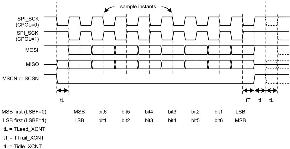
Figure 22-19. SPI Control Timing (SPICR2[CPHA]=0, SPICR1[TXEDGE]=1)
