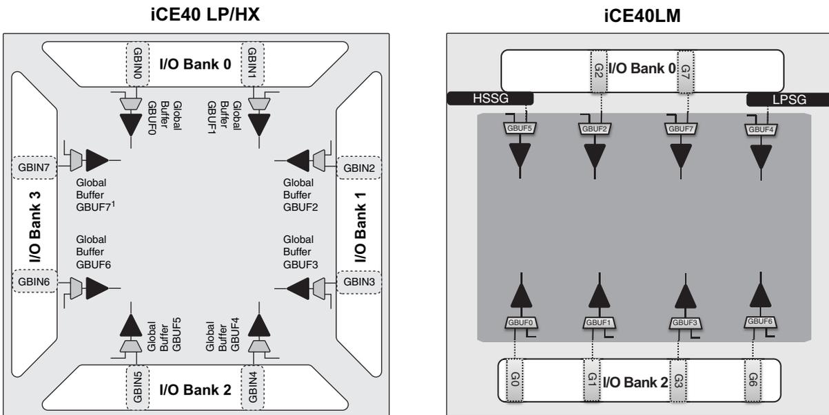
1. GBUF7 and its associated PIO are best for direct differential clock inputs.
