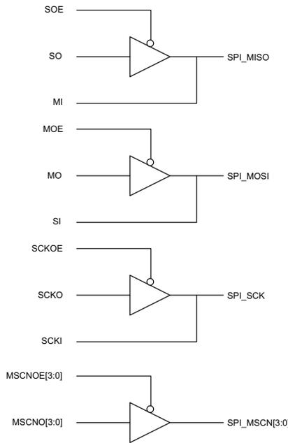
To use the dedicated SPI pins the user would start by instantiating or inferring the IO buffer. The SPI\_MISO, SPI\_MOSI, SPI\_SCK, SPI\_MCSNO[0] would then be assigned to the dedicated pins unless the dedicated pins are not available. Note the SPI pins do not have to use the dedicated pins. Refer to the diagram below for the routing connections.
