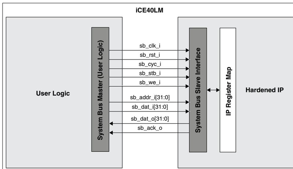
**Table 22-1. System Bus Slave Interface Signals of the Hardened IP Module**
